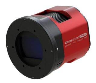
ZEUS 455C Pro cooled camera is developed by Player One, it's design for advanced DSO imaging. it adopts **Sony Industrial grade IMX455AQK-K full-frame format** color sensor. The **3.76um pixel size** accommodates a well depth of **71.6Ke** with a total of **61MP** (the resolution is 9576\*6388), and the diagonal is **43.3mm**.
