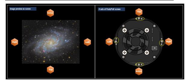
For understand 4 points adjustment method, we made an example for users:
