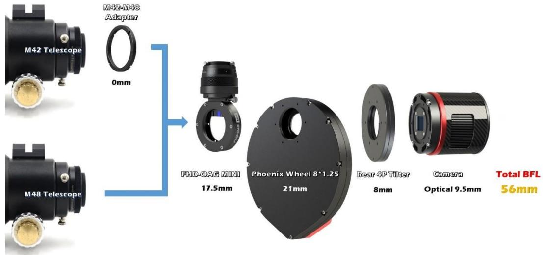
**Notice: Some BFL solution is 56mm (Compensate light path differences which caused by filters)**
