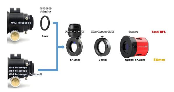
Notice: Some BFL solution is 56mm (Compensate light path differences which caused by filters)
