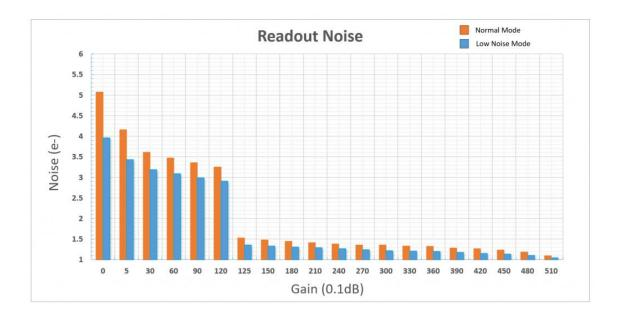
1. Normal mode has faster FPS, it is more suitable for planetary imaging.
