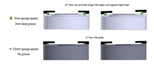
When taking solar photograph with prominence telescope, the Newton ring is annoying. Smoother solar image without Newton ring could be taken by adjusting the focal plate. Get a much smaller field curvature of the telescope.
