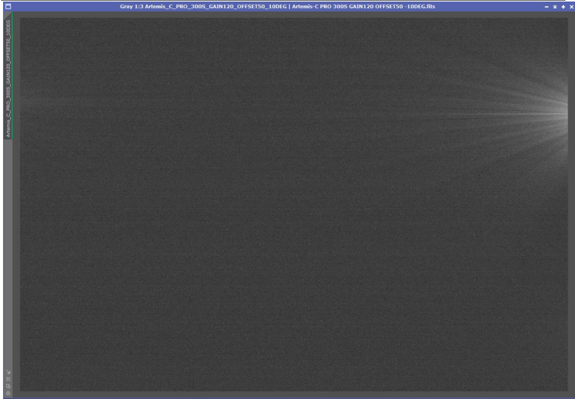
Preview of Dark frame 1: Exposure=300s, gain=120, offset=50, temp=-10°C STF auto-Stretch in Pixinsight 1.86
