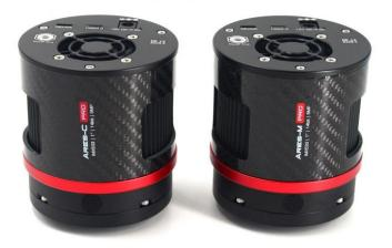
Ares-C Pro (IMX533) camera is developed by Player One Astronomy, this camera is not only great for DSO imaging, and also can do solar and lunar imaging too. Ares-C Pro camera, which adopts **Sony IMX533 1" square format** color sensor. The **3.76um pixel size** accommodates a well depth of **73Ke** with a total of 9**MP** (the resolution is 3008\*3008), and the diagonal is **16mm**.
