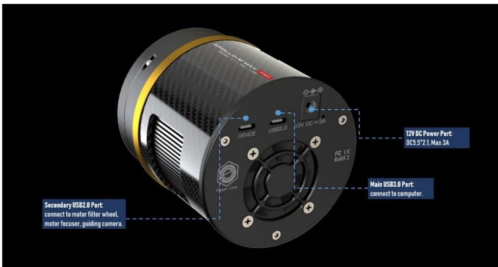
Main data port support USB3.0 protocol, type-C port is easier to plug in when assemble the imaging equipment in night. When the camera is connected to the USB3.0 interface and full-resolution preview is used, **it can reach 51FPS at 10bit(RAW8) mode and 27FPS at 12bit (RAW16) .**
